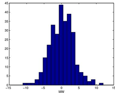
Fig. 5. Histogram of Scaled NYISO Real Time Load Deviations.
