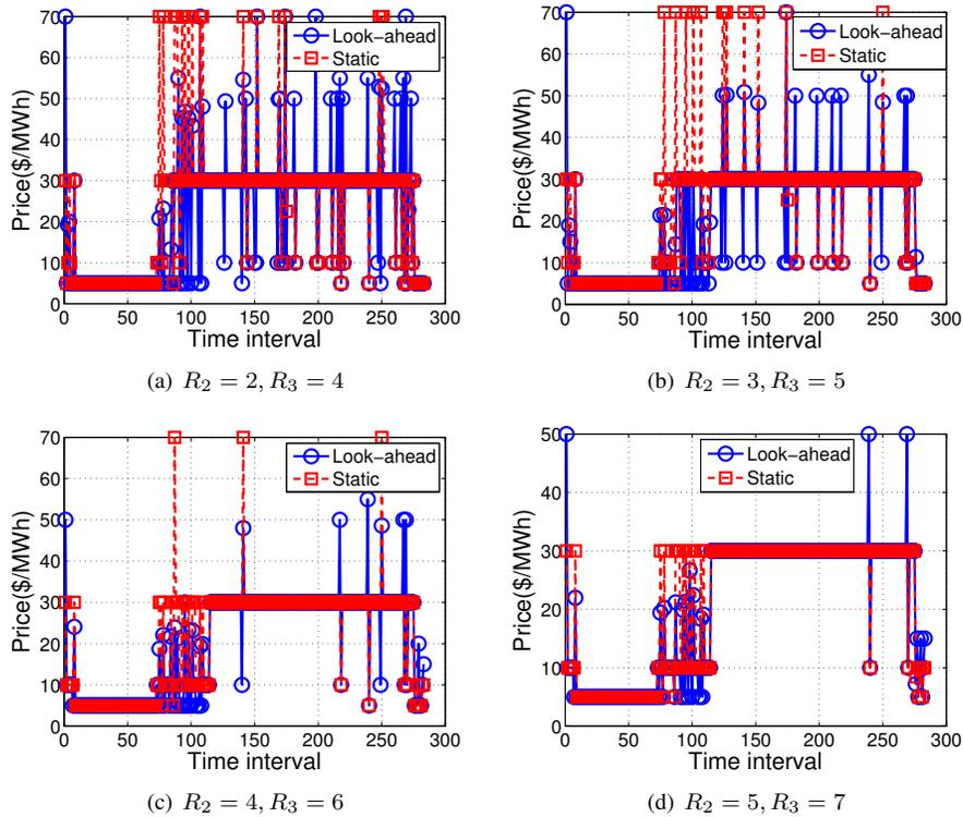
Fig. 3. Comparison of LMPs in look-ahead ( $K = 6$ ) and static ( $K = 1$ ) dispatch with varying ramp rate.
